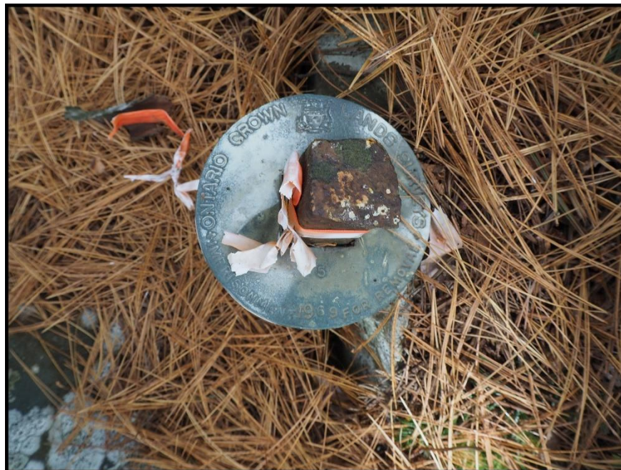
Image 21. Photograph 550 showing a second Ontario Crown Lands Survey marker in property 0108.
